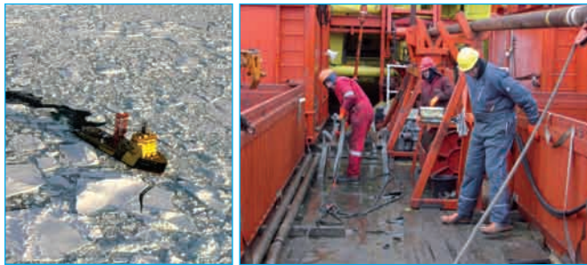
(left) Icebreaker Vidar Viking was the drilling vessel of the Arctic Coring Expedition, (right) drill rig on the Vidar Viking during coring operations (© ECORD/IODP).
