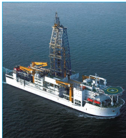
The Chikyu is a new riser drillship built by Japan, fitted with the most up-to-date technology. This 213 m-long vessel is capable of drilling in unstable area to 6-7 km below the seabed. The Chikyu started operation within IODP in 2007 in the Nankai Trough, off the east coast of Japan. By drilling into a major seismogenic zone and instrumenting boreholes to monitor long term variations of key parameters, the aim of this ambitious project is to understand what triggers devastating earthquakes and tsunamis.
