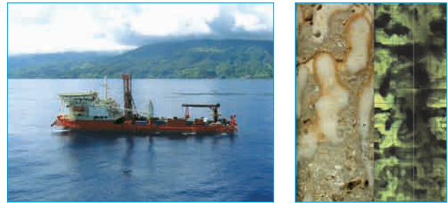
(left) Drillship DP Hunter of the Tahiti Sea-Level Expedition (right) optical borehole viewer used to examine the walls of the newly drilled boreholes to see the internal structures of the coral reefs.
