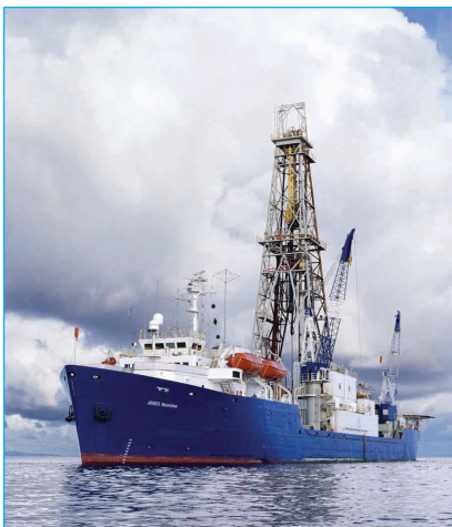
The JOIDES Resolution , the drilling vessel used during both the ODP and IODP, has proved its efficiency as a riserless vessel. It has already retrieved 333 km of cores from the seabed, and the deepest hole reaches 2,111 m beneath the seafloor. The vessel has allowed major breakthroughs in deciphering past climates, understanding Earth dynamics and documenting the deep biosphere. The JOIDES Resolution has recently undergone a major refit. Completely modernised, it will resume operations in March 2009.
