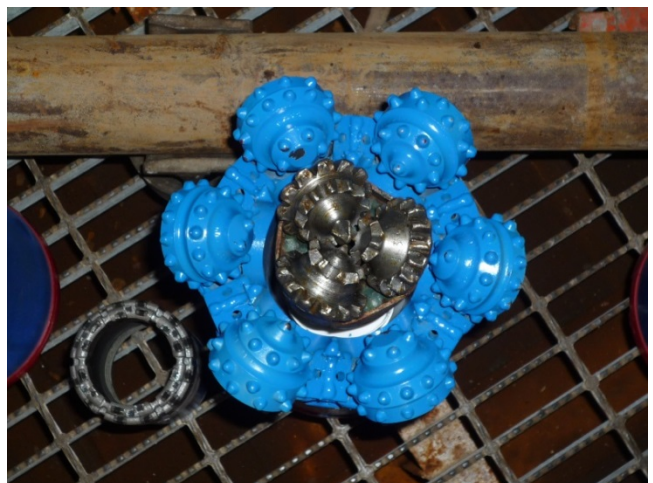
(Left) The Top Drive (yellow) in action, picking up pipes – a tank, or a Dalek? (Right) the six-cone outer roller bit (blue) with smaller inset bit (silver grey) – or is it the gaping jaws of the “Alien” ? (AnnetteMcGrath@ECORD_IODP)
