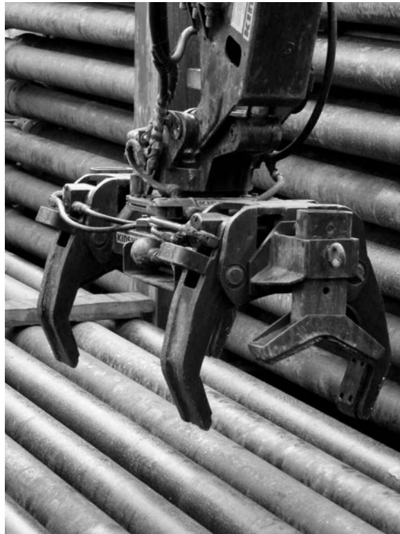
Carol Cotterill©ECORD_IODP Drill pipe waiting to be run
