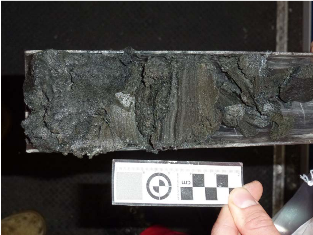
Nadine Quintana Krupinski ©ECORD_IODP Laminated muds from the core catcher sample
