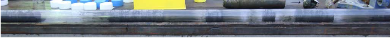
Dave Smith©ECORD_IODP Expanding 2m piston coring run in a 3.3m liner, BSB-9
