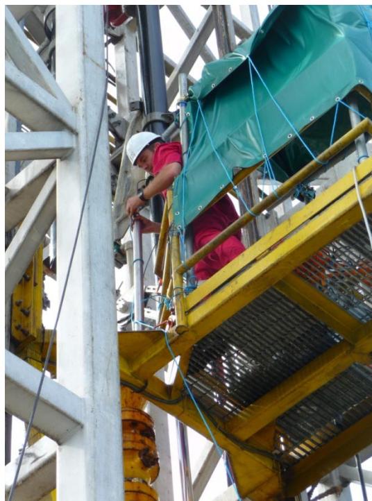
C_Cotterill@ECORD_IODP; Simon prepares to lower a probe down the drill pipe
