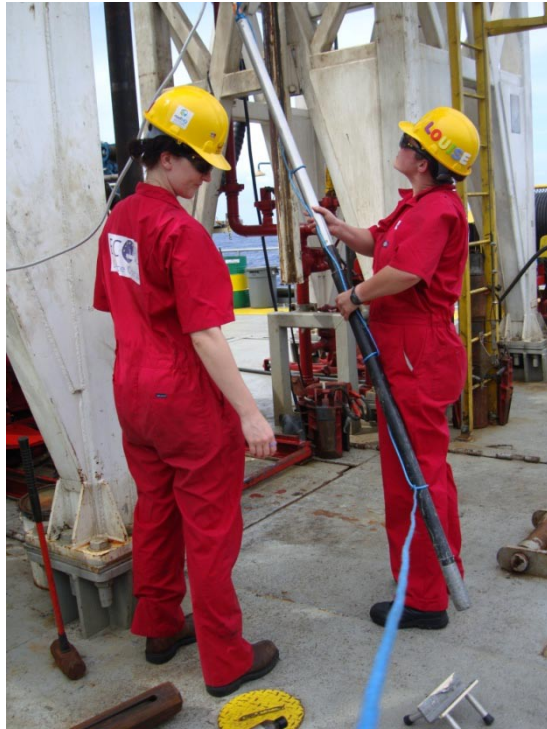
D_Smith@ECORD_IODP; Sending a probe up to the rooster box, with safety tag line attached
