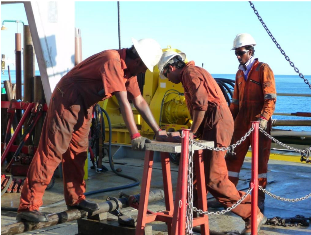
C_Cotterill@ECORD_IODP; Ajith, Vikram and Vimal “breaking” a core barrel
