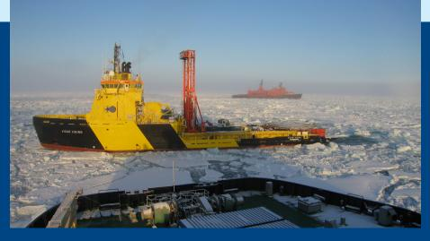
The biggest challenge during Expedition 302 was to maintain the drillship's location while drilling and coring in 2-4 m thick sea ice that moved at speeds approaching 0.5 kt.
