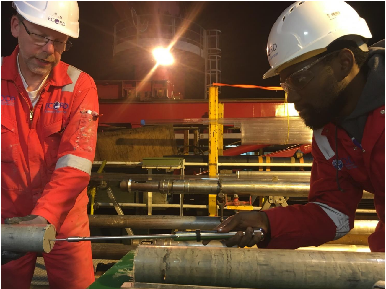
Hand-held penetrometer testing (LMcNeill@ECORD_IODP).
