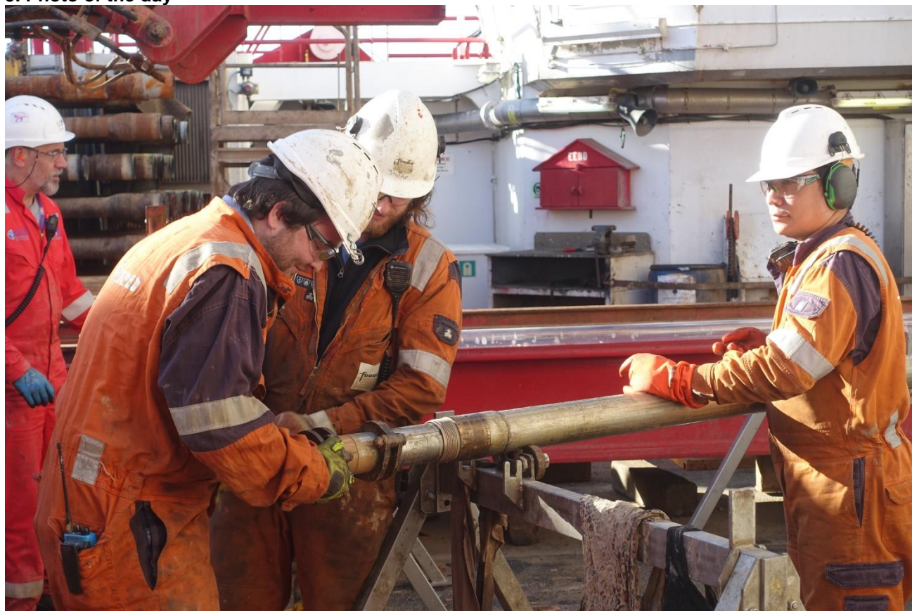
Fugro drill crew remove another core from within a core barrel (RGawthorpe@ECORD_IODP)
