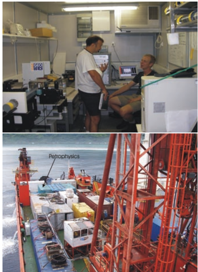
Figure 1. Offshore Petrophysics during the IODP Expedition 310 Tahiti Sea Level. The Petrophysics container is the pale blue container at the rear of the ship. The GEOTEK Multi-Sensor Core Logger (MSCL) is located within the Petrophysics container with co-chief Gilbert Camoin and Klaas Verwer (scientist).
