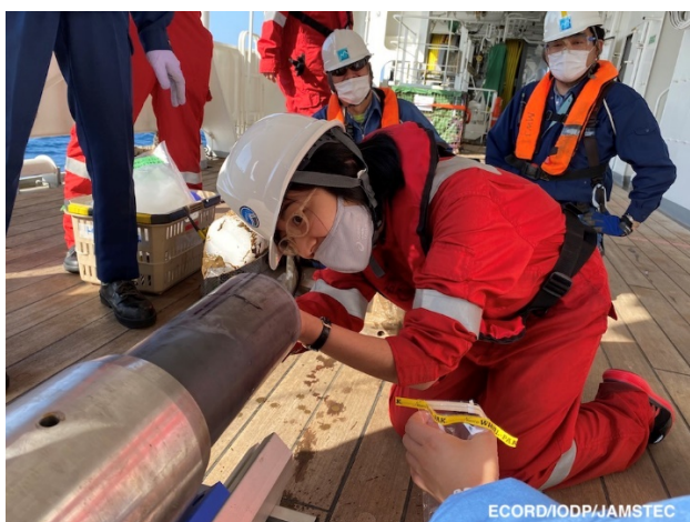
7) Kana Jitsuno collecting a sediment from the bottom of Trigger core (photo by NOKutsu@ECORD/IODP/JAMSTEC)
