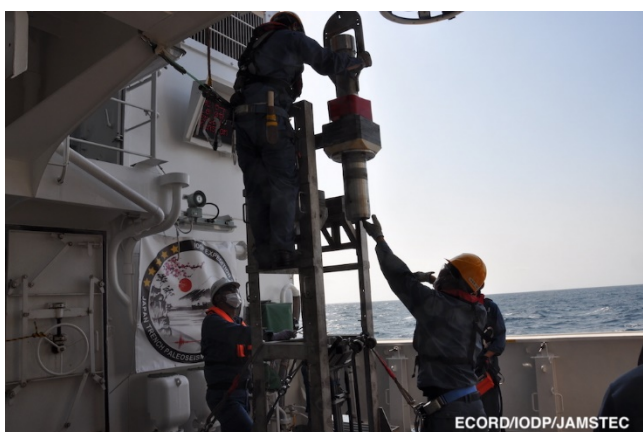
5) Removing the weighthead of Trigger corer (photo by LMaeda@ECORD/IODP/JAMSTEC)
