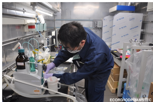
8) A lab tech preparing auto-titrator (photo by LMaeda@ECORD/IODP/JAMSTEC)
