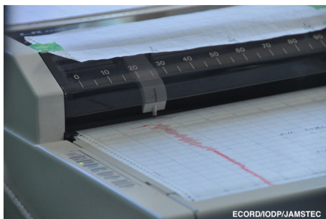
2) A pen recorder showing spud-in and release (photo by LMaeda@ECORD/IODP/JAMSTEC)
