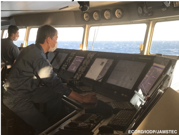
1) Captain himself operating DPS by manual mode (photo by LMaeda@ECORD/IODP/JAMSTEC)
