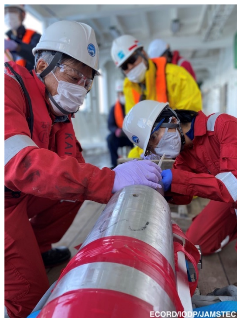
8) Microbiology specialist Kana Jistuno taking sediment samples from Trigger core (photo by NOkutsu@ECORD/IODP/JAMSTEC)
