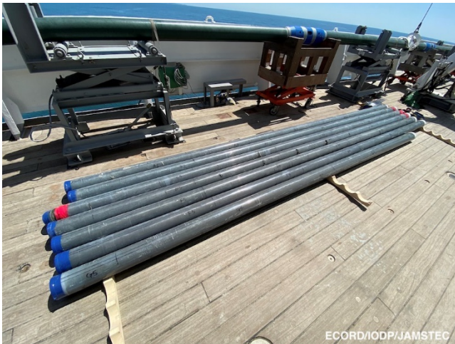
2) 5 m core segments waiting for cutting into 1 m sections (photo by NOkutsu@ECORD/IODP/JAMSTEC)
