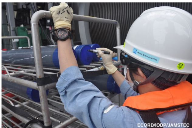
4) Curatorial staff marking section ID on a top end cap (photo by LMaeda@ECORD/IODP/JAMSTEC)
