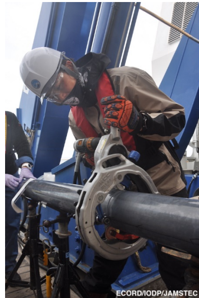
2) Assistant offshore EPM Nori Sakurai cutting core into 1 m sections (photo by LMaeda@ECORD/IODP/JAMSTEC)
