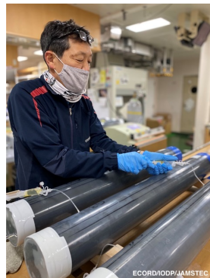
5) Scientist Toshiya Kanamatsu collecting IW using Rhizon sampler (photo by NOkutsu@ECORD/IODP/JAMSTEC)
