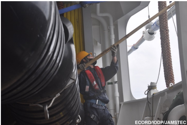
1) A deck crew propping up the core barrel with a bamboo pole (photo by LMaeda@ECORD/IODP/JAMSTEC)
