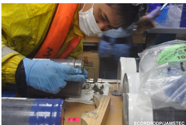
4) A lab tech attaching "patch" on an expanded core section (photo by LMaeda@ECORD/IODP/JAMSTEC).
