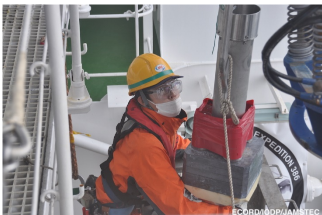
3) A deck crew removing Trigger weighthead from the core barrel (photo by LMaeda@ECORD/IODP/JAMSTEC)
