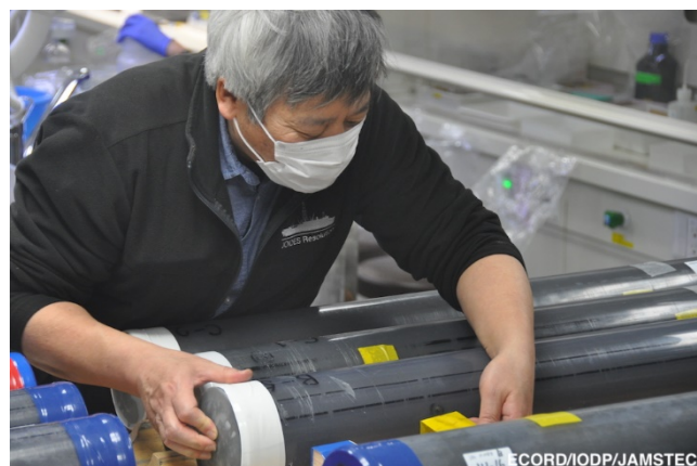
5) Co-Chief Ken Ikehara checking a drilled hole for gas expansion in the core, tapping the base to encourage release (photo by LMaeda@ECORD/IODP/JAMSTEC)
