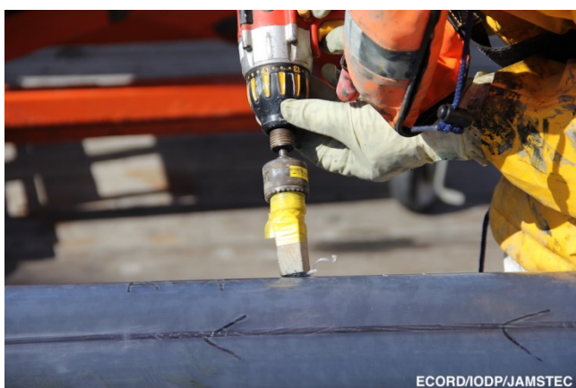
5) Drilling a hole in the liner to release gas pressure (photo by LMaeda@ECORD/IODP/JAMSTEC)
