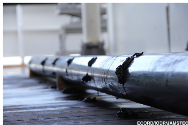
6) Mud snakes everywhere caused by gas expansion (photo by LMaeda@ECORD/IODP/JAMSTEC)
