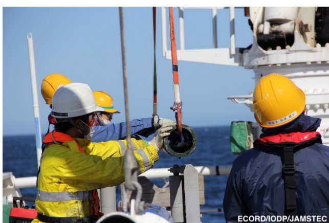
4) Deck crew removing the bottom barrel using a crane (photo by LMaeda@ECORD/IODP/JAMSTEC)
