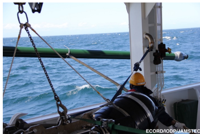
2) A deck crew member catching the barrel with a bamboo pole (photo by LMaeda@ECORD/IODP/JAMSTEC)
