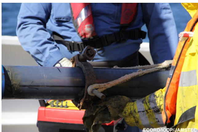
3) The clamp to help withdraw the liner (photo by LMaeda@ECORD/IODP/JAMSTEC)
