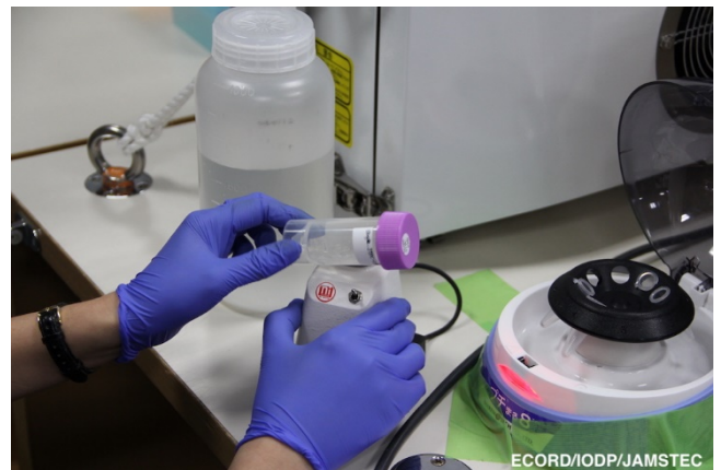
3) Vibrating a sample before observation under microscope (photo by NOKutsu@ECORD/IODP/JAMSTEC)
