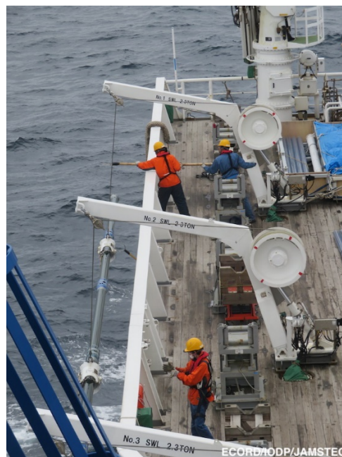
2) Recovering the barrel string to the deck (photo by Kikihara@ECORD/IODP/JAMSTEC)
