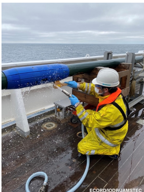
3) Washing the barrel coupler (photo by NOkutsu@ECORD/IODP/JAMSTEC)
