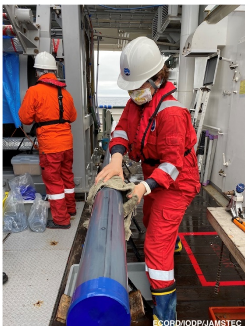
4) Offshore EPM Lena Maeda wiping the core clean (photo by NOkutsu@ECORD/IODP/JAMSTEC)
