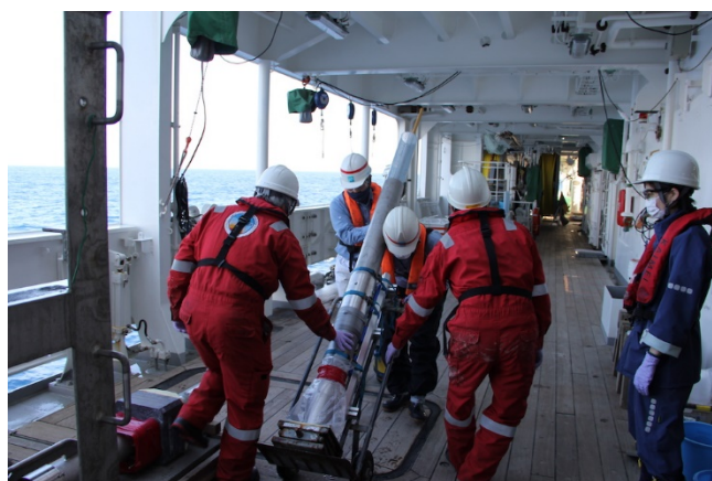
2) Laying down the Trigger corer for cutting core liner and sampling (photo by LMaeda@ECORD/IODP/JAMSTEC)
