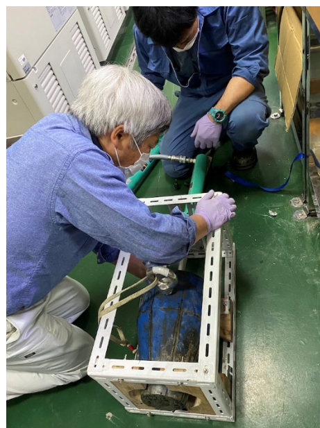
4) Co-Chief Ken Ikehara setting a core bit on a hydraulic pusher (photo by NOkutsu@ECORD/IODP/JAMSTEC)
