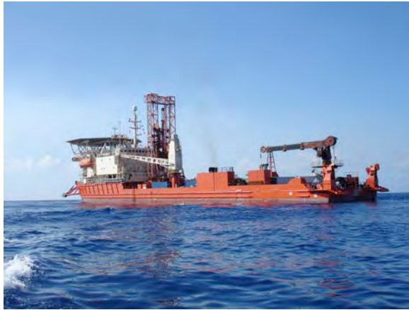
The DP Hunter coring off Tahiti. Photo: I Pheasant© IODP/ECORD
