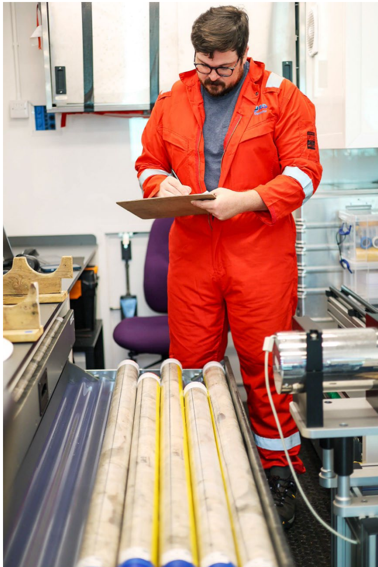
Photograph by Marley Parker © ECORD_IODP. Physical Properties Specialist Brian Boston assessing cores from M97B prior to MSCL logging.
