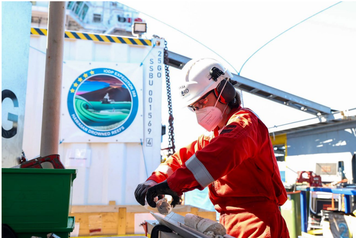
ESO Assistant Lab Manager and Curator Patrizia Gepraegs transferring core samples cored in an aluminium liner to a plastic liner during on-deck core curation. Photo by MarleyParker@ECORD_IODP.
