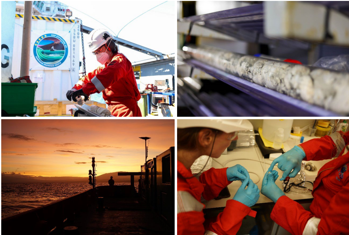
Clockwise from top left: ESO Assistant Lab Manager and Curator Patrizia Gepreags transferring core samples cored in an aluminium liner to a plastic liner during on-deck core curation. Photo by MarleyParker@ECORD_IODP. Core on deck. Photo by MarleyParker@ECORD_IODP. Processing of geochronology and aDNA samples by the geochemistry team. Photo by ELB@ECORD_IODP. Observing a stunning sunrise over Big Island. Photo by ELB@ECORD_IODP.
