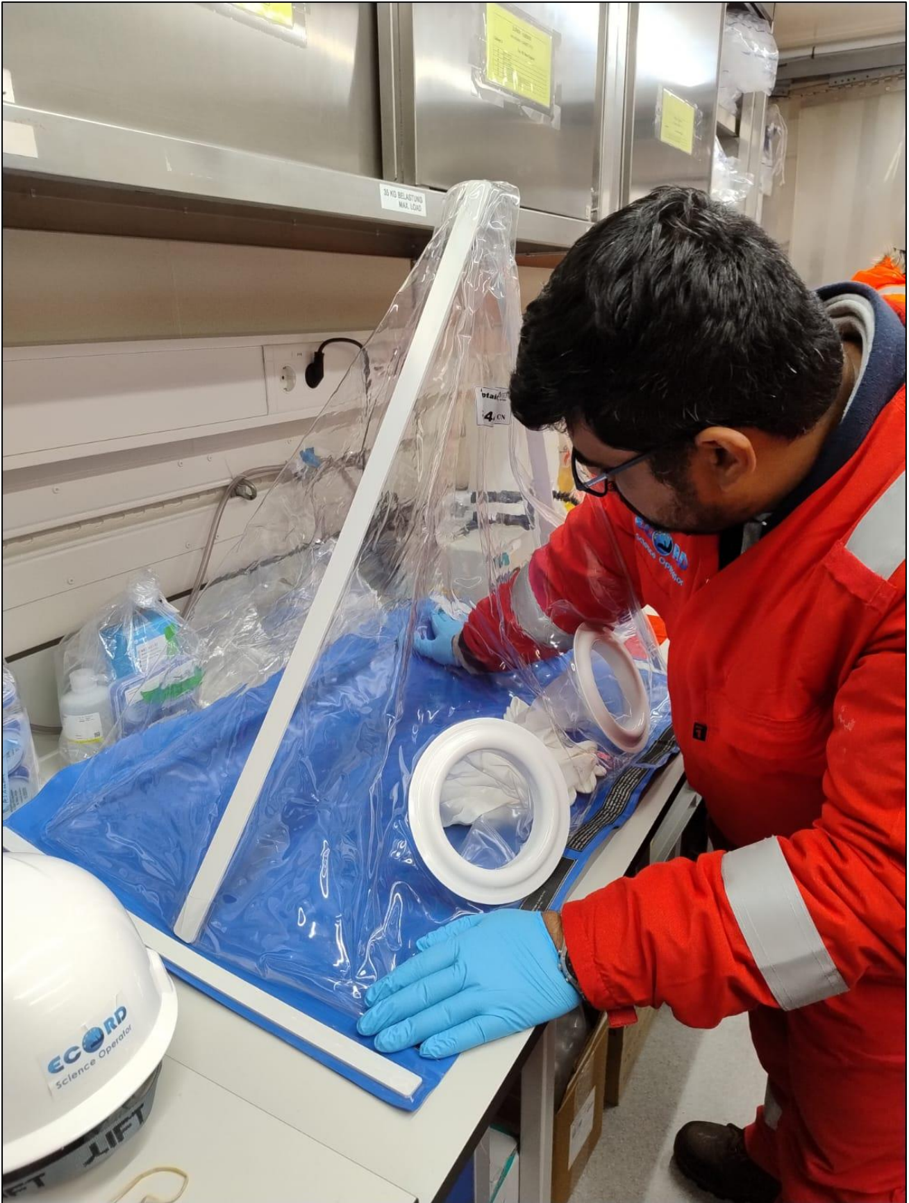
Expedition 501 scientist Avishek Dutta cleans the portable glove bag inside the Geochemistry Container in preparation for taking microbiology samples. STEWART@ECORD_IODP3_NSF_Dutta_glove_bag
