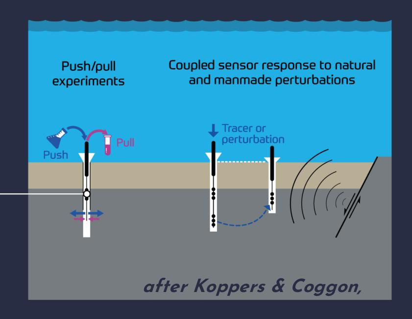
We can conduct subseafloor experiments
