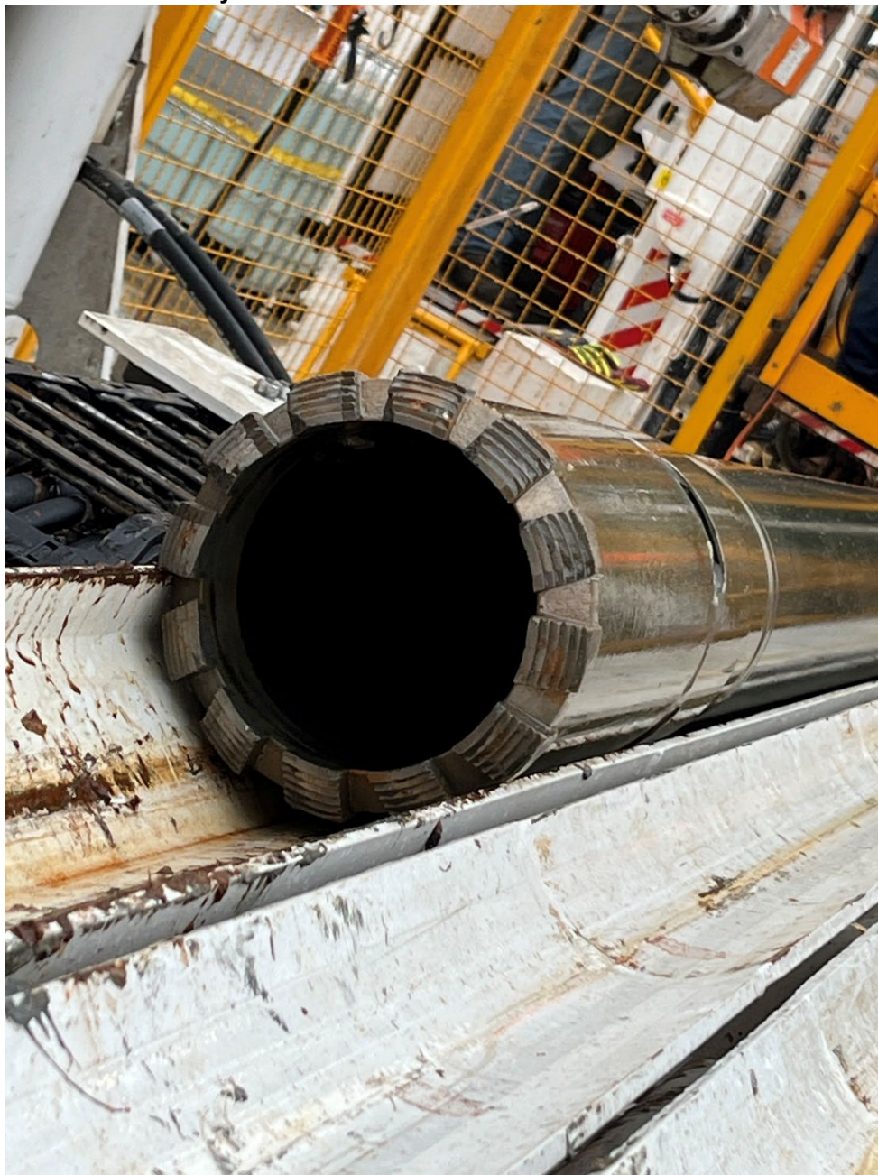
Figure 1: 6 5/8" casing shoe, back on deck after the conclusion of M0111-B (photo BARBOSA@ECORD_IODP3_NSF_Casing_Shoe).
