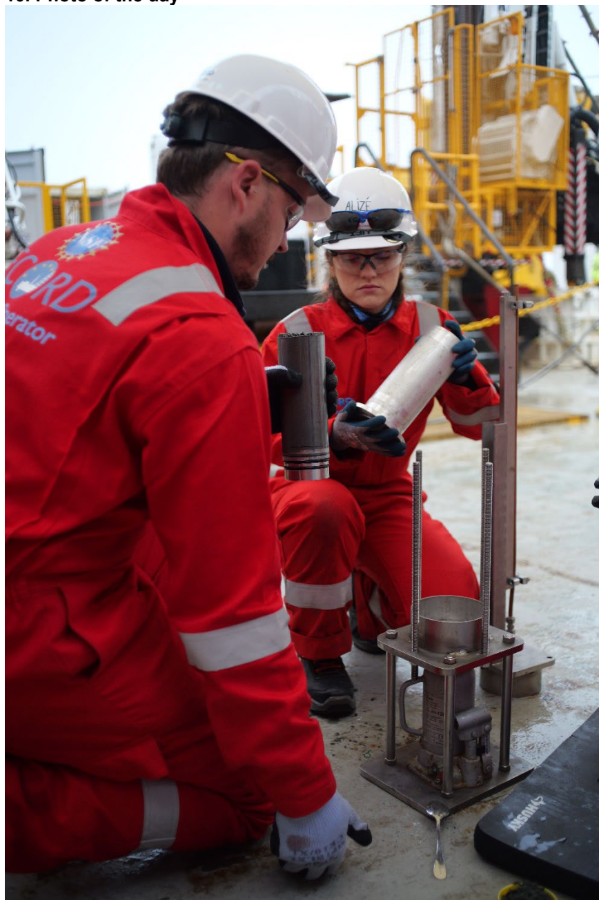
Figure 1: Preparing equipment for sampling of sediments for noble gas analysis (photo LEBER@ECORD_IODP3_NSF_NG_sampling2).
