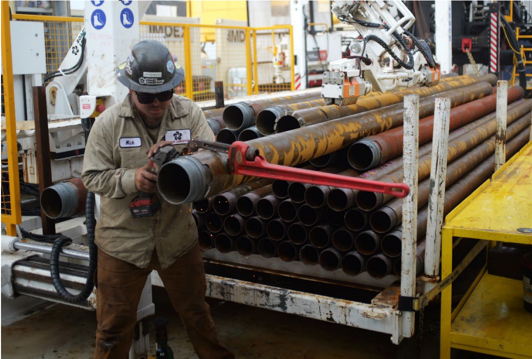
Figure 1. Nick McMahon from Boart Longyear, cutting the joining lugs from the casing (LEBER@ECORD_IODP3_NSF_rigfloor).
