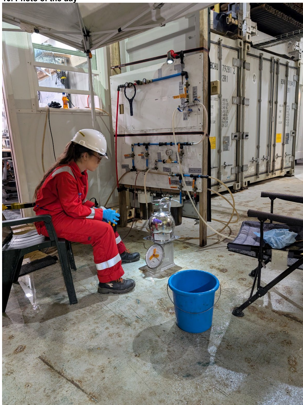
Figure 1: Science Team member Alizé Longeau filling vacuum flasks with samples for analysis of noble gases Argon, Krypton and Xenon (photo GEPRAEGS@ECORD_IODP3_NSF_Noble_Gas_Sampling ).
