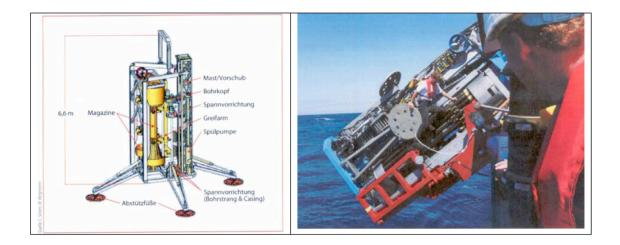
In Figure: the portable seafloor drill rig Meeresboden-Bohrgerät (MeBo) represent the newest advance and innovation in marine drilling technology at *European dimension*.
