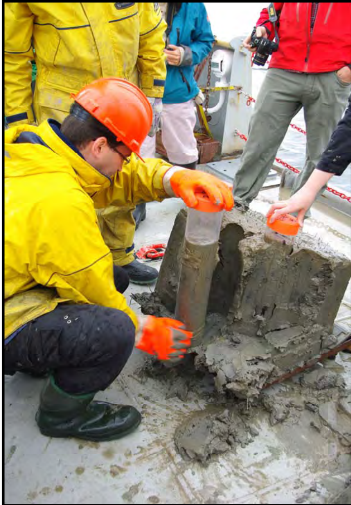
Guillaume in photo showing push core COR1003-03-BC being removed from the box core and sealed shut with plastic caps.
