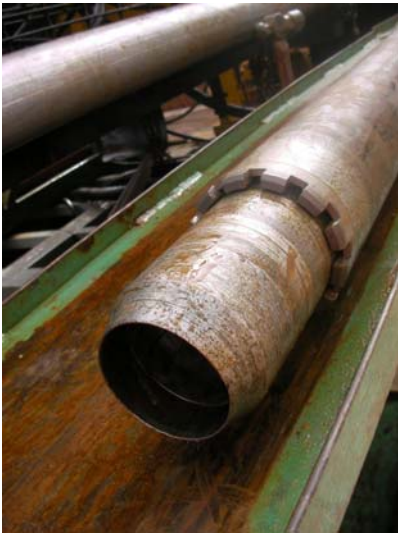
Photo 2. Graham Tulloch. The extended nose corer, one of the drill bits used in this Expedition.
