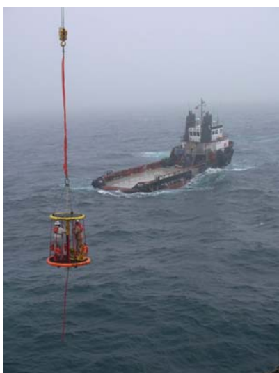
David McInroy. 1 st May. The supply vessel Rana Miller arrives at the L/B Kayd to drop off equipment and personnel. The transfer between the Rana Miller and L/B Kayd is done by hoisting a small platform (the 'Billy Pugh', foreground) between the two platforms.
