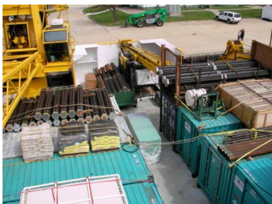
David McInroy. 30 th April. The working deck of the L/B Kayd . The drill rig mast is down in preparation for transit. Stacks of drill pipe are secured, and the various ESO container laboratories are arranged in a street-like formation.
