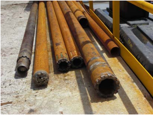
A selection of coring tools. From left to right: extended nose corer, full-face insert bit, ALN rotary corer (x2), outer drill bit. The 4 coring tools on the left fit into the outer drill bit to form the bottom hole assembly, which drills out the sediment and cuts the core ( Carl Peters©ECORD/IODP ).
