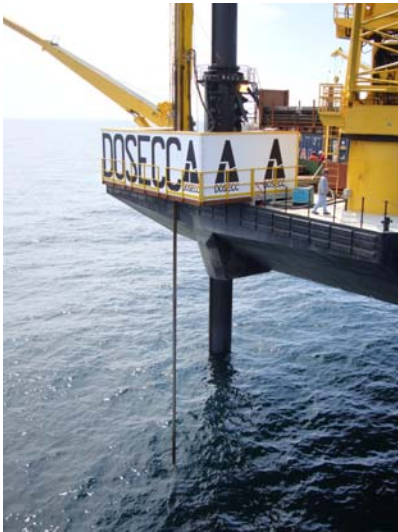
The drill rig, which hangs over the bow of the L/B Kayd , lowers the drill string into the sea bed ( Dave Smith@ECORD/IODP ).
