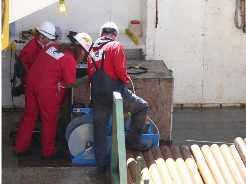
Photo 2. Wireline Logging underway, with Vanessa, Jenny and Simon. Our job is two fold. We carry out our observations with both a technical and scientific eye. Whilst operating the winch, not only do we have to make sure that all is functioning properly mechanically and electronically, but more importantly we have to verify and validate the quality of the data as the measurement is made. (Photo: Susanne Stadler©ECORD/IODP).
