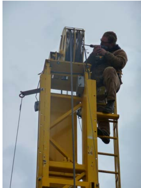
C_Cotterill©ECORD_IODP – Chris Delahunty, DOSECC, attaches the wireline counter with newly installed circuit board to the drilling rig
