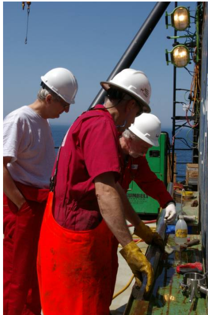
Photo 1. Measuring the core in 1.5m sections prior to entry into the DIS. (J Gafeira©ECORD/IODP)
