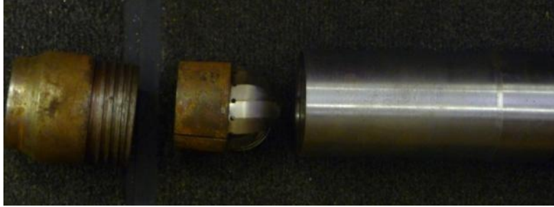
Shoe, core spring basket catcher combination and inner core barrel(C.Cotterill©ECORD/IODP).
