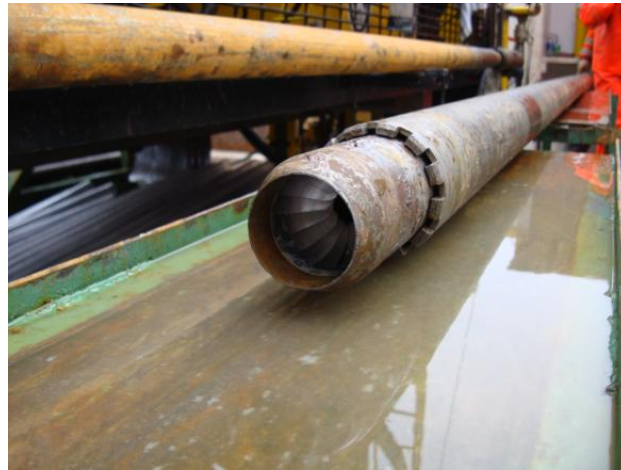
Diamond impregnated bit with shoe and basket catcher. (D. Smith©ECORD/IODP).
