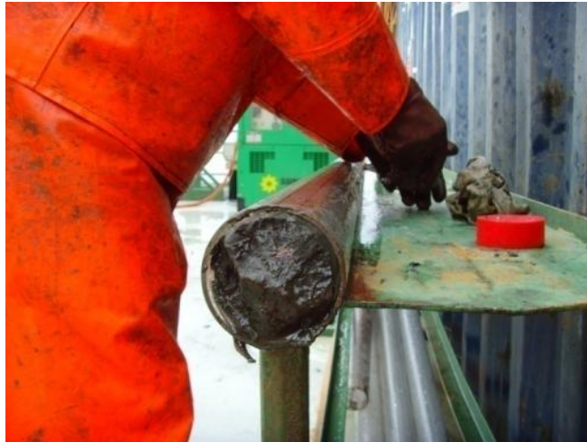
Capping the core as it arrives on deck ( J. Inwood©ECORD/IODP ).
