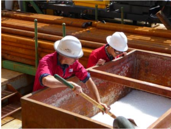
Graham Tulloch (ESO Drilling Coordinator) shows Takeshi Hayashi the mud mix in the tanks, while Jess (DOSECC) mixes up another batch of Guar Gum (C.Cotterill©ECORD/IODP).
