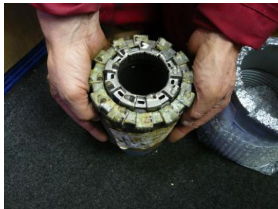
PCD PQ bit and PCD ALN coring bit and tungsten carbide casing shoe (to the right in the picture (E. Gillespie©ECORD/IODP).
