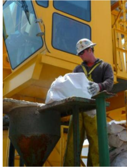
Graham Tulloch (ESO Drilling Coordinator) shows Takeshi Hayashi the mud mix in the tanks, while Jess (DOSECC) mixes up another batch of Guar Gum (C.Cotterill©ECORD/IODP).
