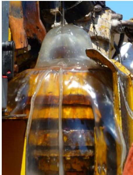
Retrieving the core barrel often pushes a fountain of drilling fluids ahead of it! (C.Cotterill©ECORD/IODP).
