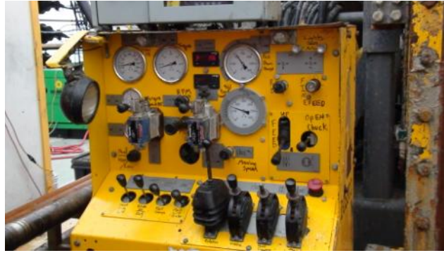
Control panel on the drilling rig showing the many dials and levers the drilling crew monitor constantly for water pressure, torque, pullback and pushdown pressure on the drill bit and mud supply rates amongst other things (D.McInroy©ECORD/IODP).
