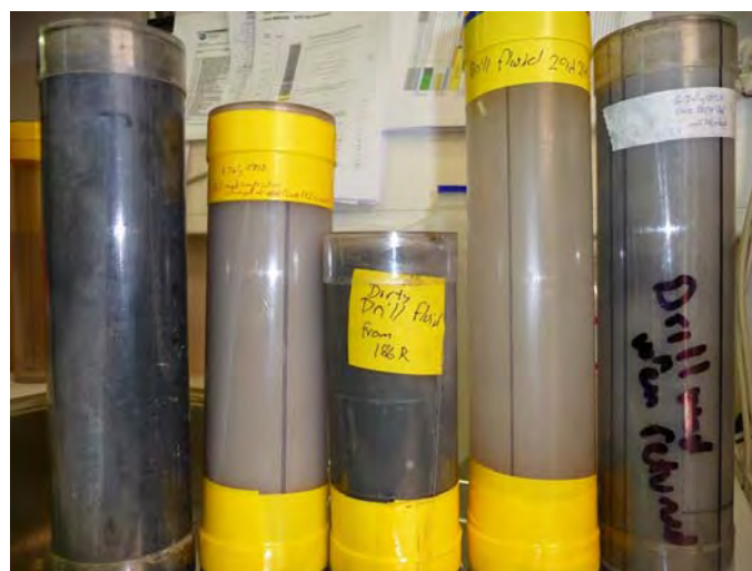
C_Cotterill©ECORD_IODP_Different drill fluid mixes have their physical properties measured as baselines
