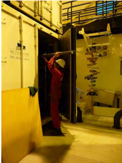
C_Cotterill©ECORD_IODP_The core now goes into the reefer to cool before MSCL measurements are taken
