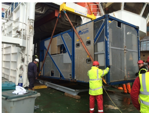
Marum MeBo winch being installed. ©Dave Smith
