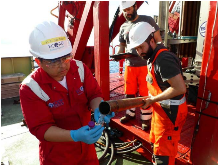
Sampling the drill liner fluid for PFC Tracer analysis. DaveSmith@ECORD_IODP
