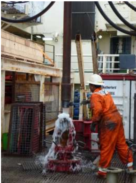
Yaya greases a pipe before adding to the string
