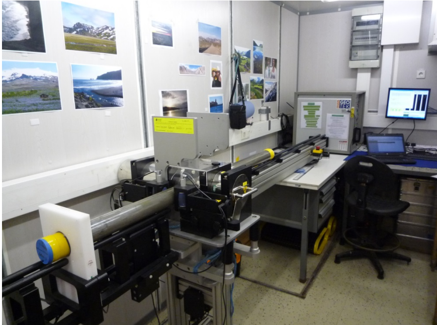
The Geotek Standard MSCL logging core in the Petrophysics Container. Photo AnnetteMcGrath@ECORD_IODP
