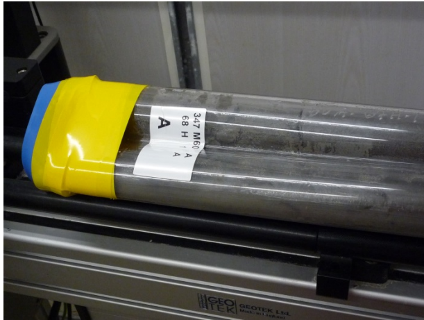
(Left) A squashed "banana" core. (Right) A large section of a metal core catcher within the core liner - it produced some interesting magnetic susceptibility results. (Photo on the left Photo AnnetteMcGrath@ECORD_IODP Photo on the right AnneSophieFanget@ECORD_IODP).
