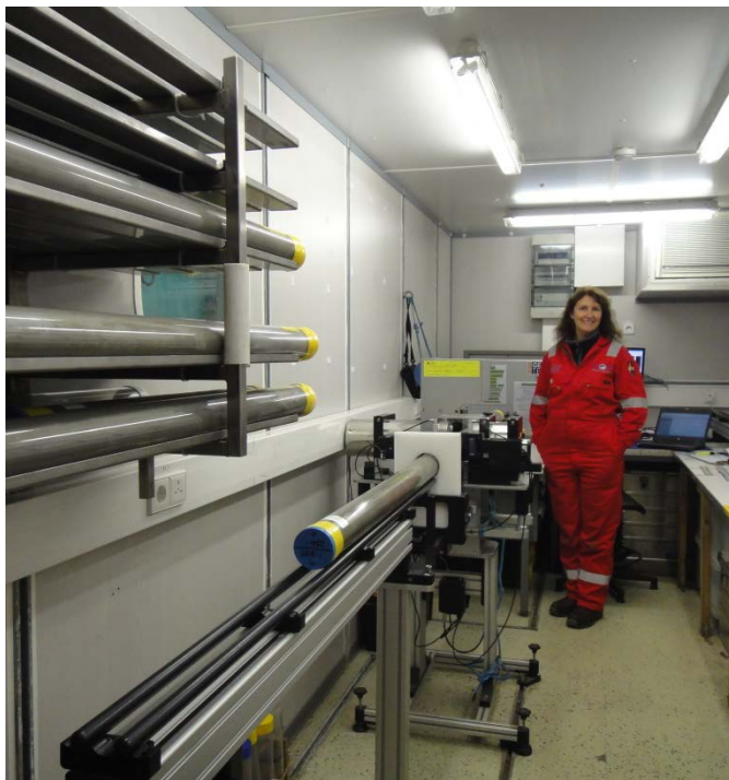
The Standard MSCL (left) with a core moving through the magnetic susceptibility loop, and (right) I just love the Fast-Track MSCL (Both photos MaryMowat@ECORD_IODP).
