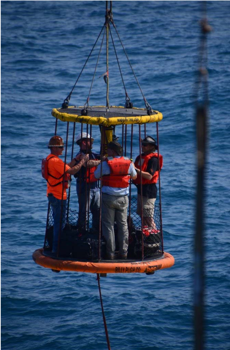
Photograph by Chris Lowery © ECORD/IODP Scientists transfer to the L/B Myrtle via a Billy Pugh
