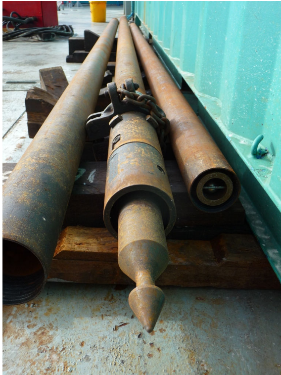
C_Cotterill@ECORD_IODP; View of the latchhead – the top of the sample tube, onto which the overshot latches to pull it back up
