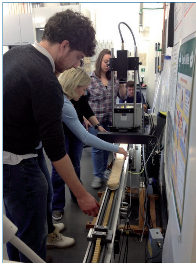
ECORD Training School: early-career scientists learn how to operate the Multi Sensor Core Logger (MSCL) (photo Ursula Röhl/MARUM).
