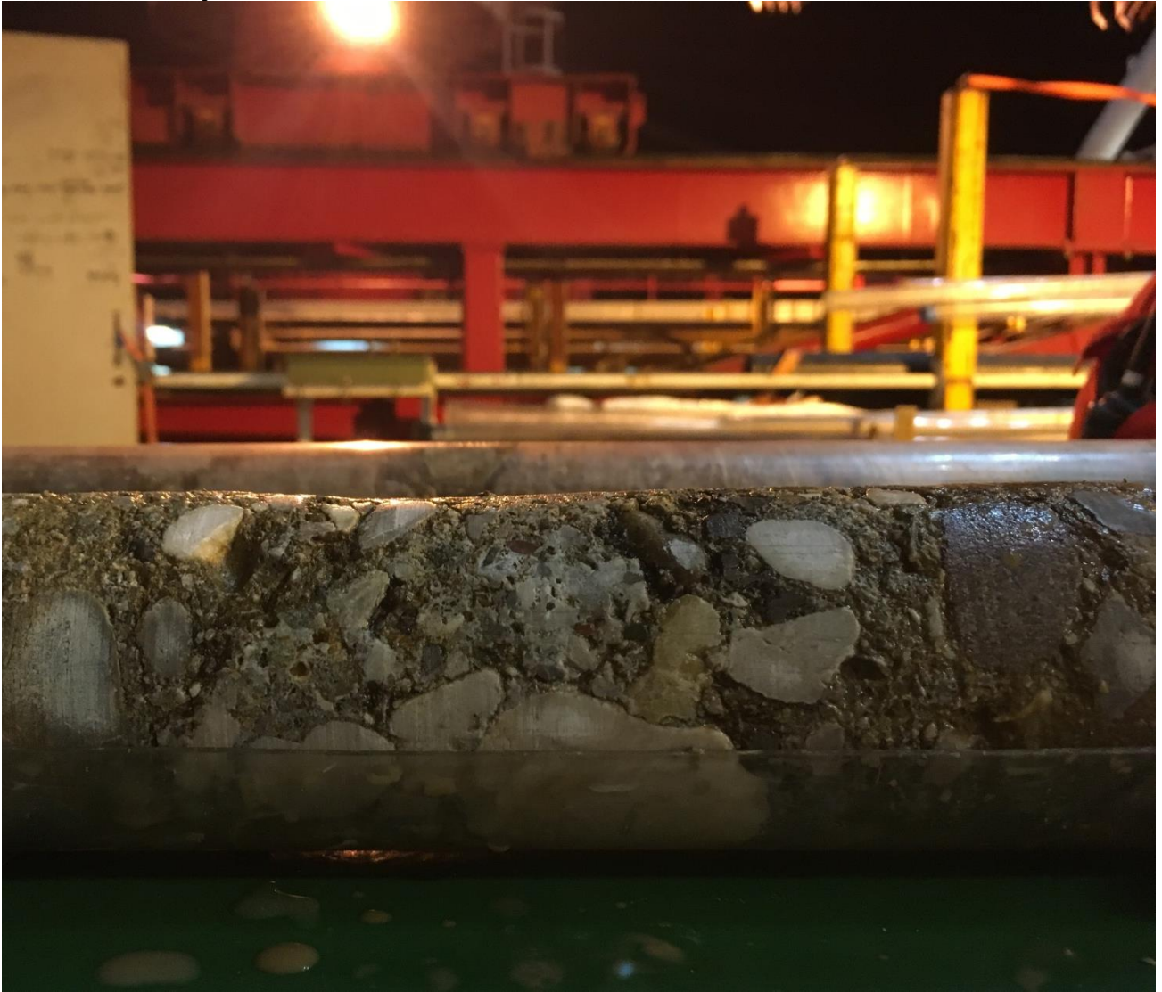
Basal conglomerates were encountered in the final cores of Hole M0080A (LMcNeill@ECORD_IODP)
