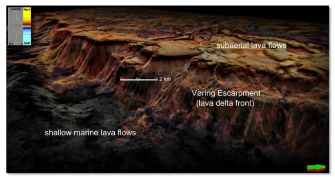
Amplitude map of the surface of the extruded magmas on the Vøring Margin. The image shows an approximately 80 km-long segment of the Vøring Escarpment buried beneath several hundred meters of sediments. This data example illustrates the power of modern 3D seismic data in selecting drilling targets in a volcanic province. The arrow indicates north. Data courtesy: Chevron. Image by A. Groth, Statoil.
